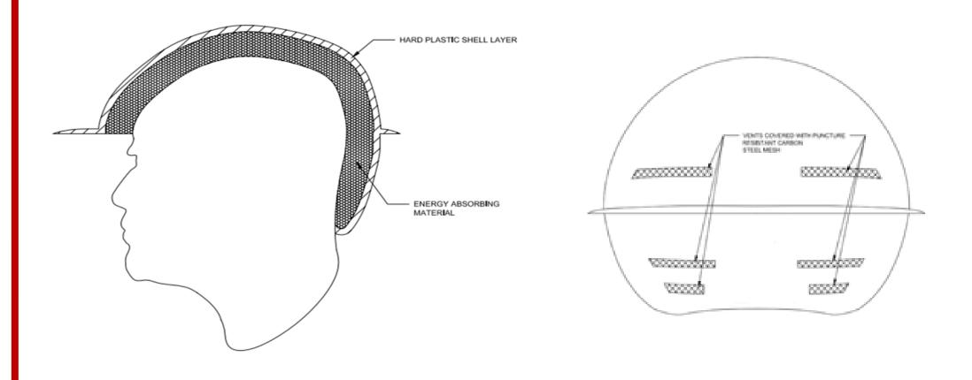
**Outer Shell:** Final prototype consists of ABS material
