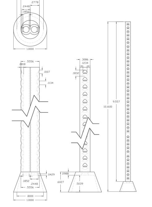
The material used to create this piece is VeroClear RGD810. The material used for the testing strips is foam coated with the reagents needed to cause a color change when in contact with Leukocytes or Nitrites in the urine. In order to have the time release function and allow the CAUTI detector to last up to 8 hours, the entire device is coated with Surelease® Ethylcellulose Dispersion Type B NF.
