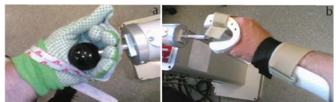
Fig. 1. a. Glove attached to the end effector of the Haptic Master. b. For more involved subjects, a commercial resting hand splint was attached to the end-effector of the Haptic Master via ball and socket joint.
