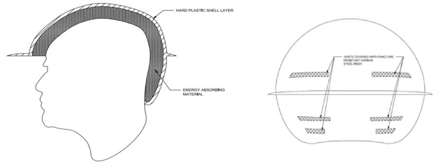
**Outer Shell:** Final prototype consists of ABS material
